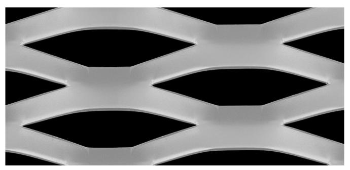
LW Pitch:135.00mmStrand Width:15.00mmSW Pitch:42.00mmThickness:3.00mmWeight:5.78 kg / m2Open Area:28%
